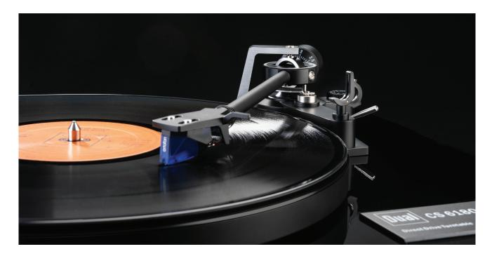
winit in the similarly priced Technics SL1500C, it doesn't feel as hefty, an impression partly created by the Dual running on a 12v wall wart rather than having a mains input. Nevertheless, the spin up time is extremely brisk and the CS-618Q gives you the option of 33, 45 and 78rpm playback. The platter it acts on is cast aluminium and damped via 2.5mm thick rubber mat.
